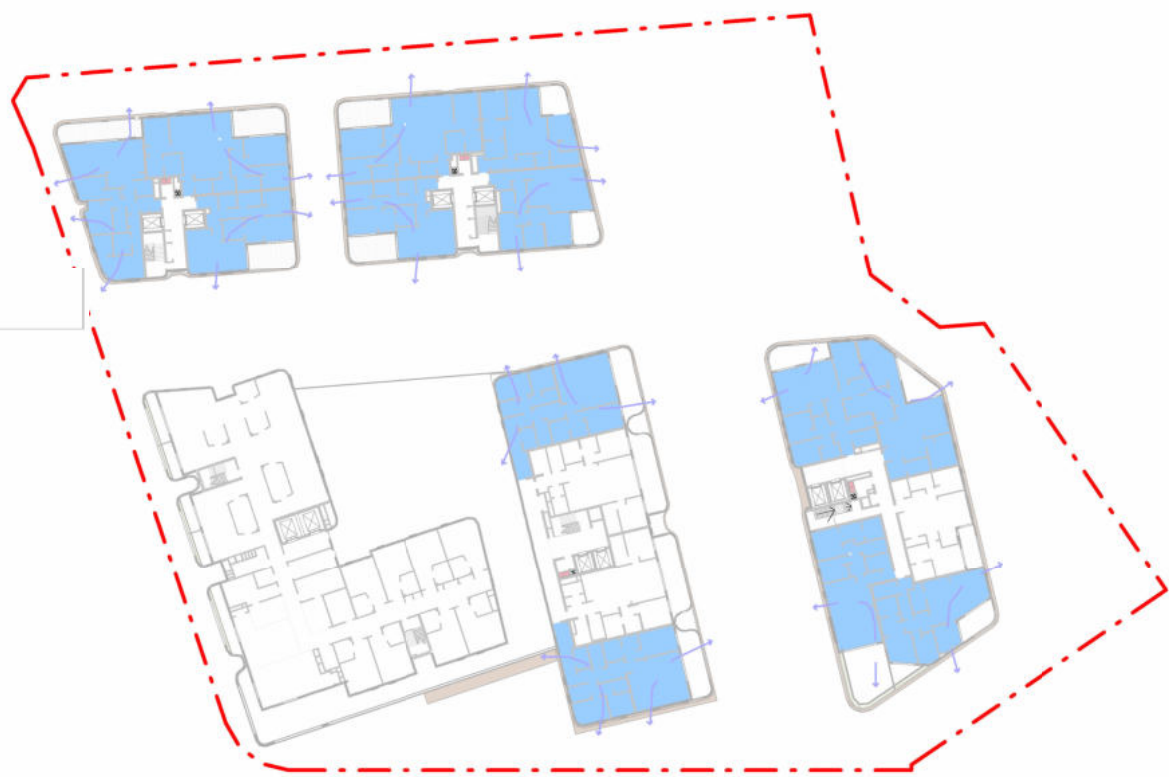
2 LEVEL 1 OVERALL FLOOR PLAN CROSS VENTILATION 1 : 1000
